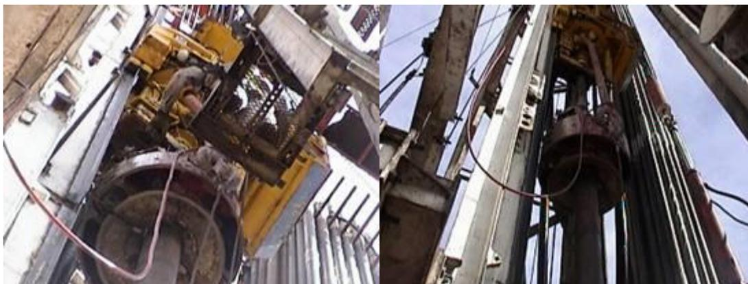
Heavy Weight Casing Elevator. Heavy Weight Casing Elevator.
